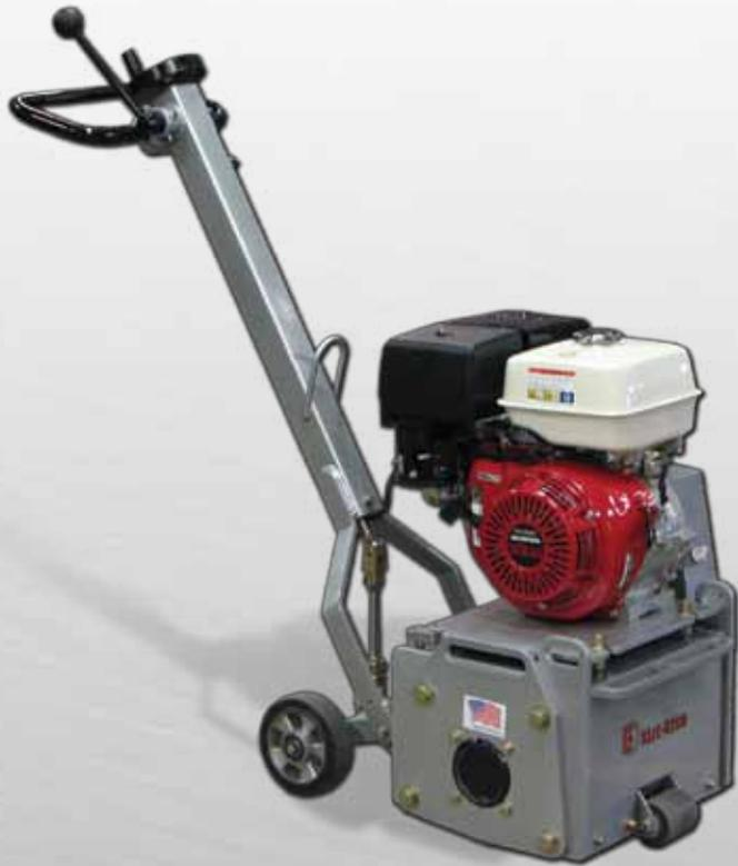
The KR13 (13-inch cutting path) is the epitome of heavy-duty scarifier machinery. It offers approximately 423 pounds (with drum) of centrally located quality engineering that refuses to "jump out of the cut." It is offered in three models: The 11-horsepower gas-driven, the 13-horsepower gas-driven and the 5-horsepower electric.
